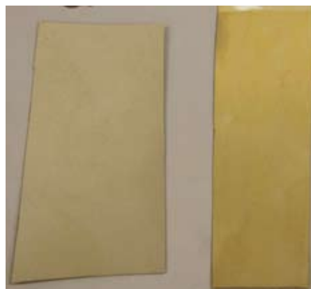
Figure 4 A typical vinyl copolymer silver ink pattern before and after heat and humidity exposure
