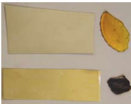
Figure 6 The base polymer used in the ink before and after humidity exposure
